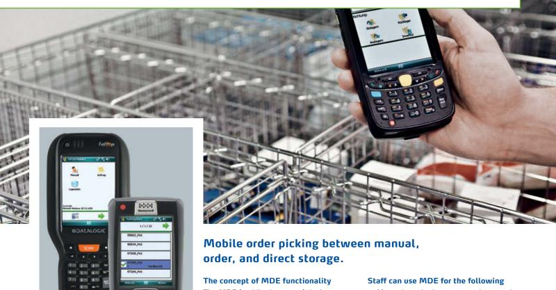
The MDE (mobile data entry) device replaces the stationary Power Pick Global workstation, which is operated with dynamic storage systems, such as Shuttle XP and Megamat RS. It is used in applications where the goods are not brought to the person.
