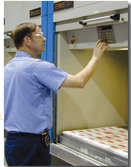
Operator uses the operator friendly keypad to enter a tray number for retrieving or putting away a part.
